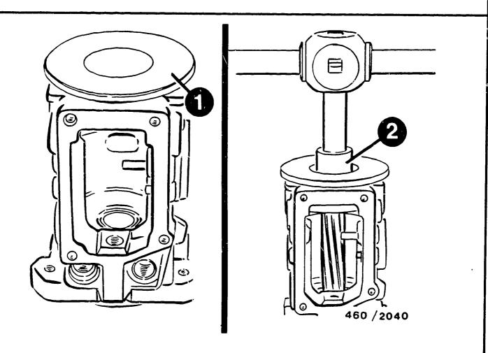
Attach wrench to reamer and ream inner bushing with oil.
